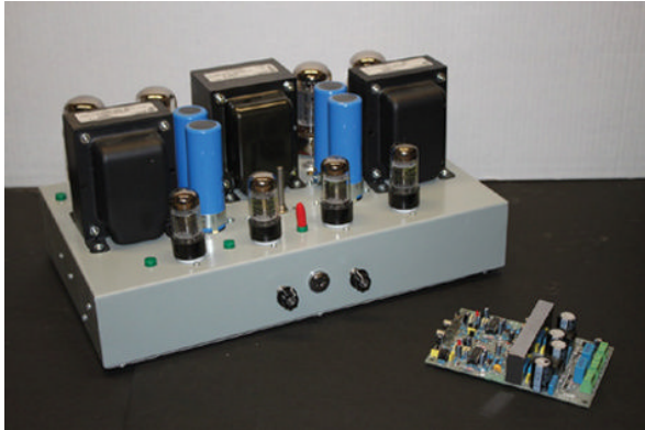
FIGURE 1.1 A comparison: Vacuum-tube audio amplifier (left) using a design circa 1955 and class D amplifier (right) using a design circa 2008.
