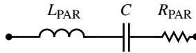
FIGURE 3.3 Equivalent circuit of capacitor showing parasitic inductance L_{PAR} and equivalent series resistance R_{PAR} in series with capacitance C .
