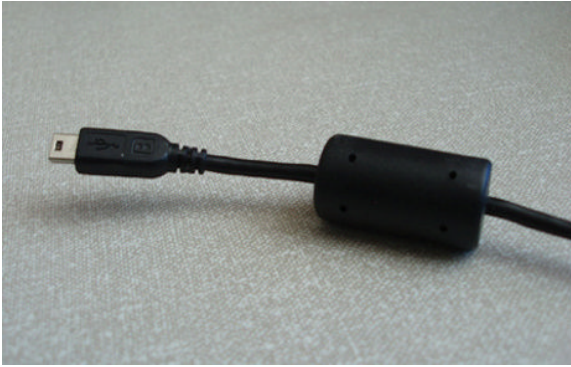
FIGURE 11.8 Ferrite-choke RFI filter on USB cable carrying digital signals.
