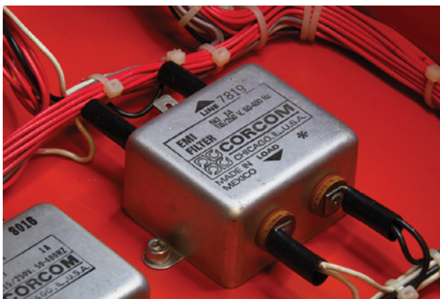
FIGURE 12.14 AC power-line EMI filter packaged in shielded metal case.
