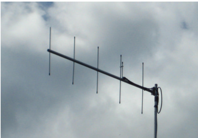
FIGURE 11.36 Yagi antenna used to produce moderately directional beam of radio waves. The entire antenna is about 0.3 m (1 ft) long.
