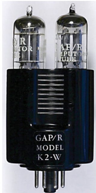
FIGURE 5.1 The first commercially available operational amplifier used two vacuum tubes and cost $24 in 1952. (From www.PhilbrickArchive.org . Reproduced by permission of Joe Sousa.)
